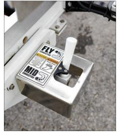
**WATERWAY CONTROLS:** Repositioning the waterway can be done easily with the flip of a mechanical lever. Available on Ladder Tower aerials.
