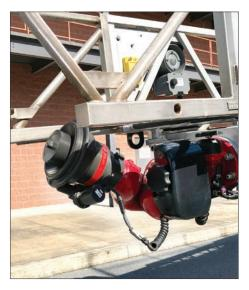
**WATER MONITOR:** When positioned at the tip, the water monitor can be set to reach 30° higher than the elevation of the ladder.
