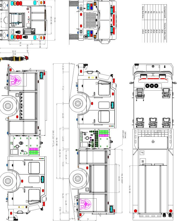
WATER/FOAM: 750 GALLONS / 20 GALLONS ΔXLES: ENERATOR: OAM SYSTEM: RANSMISSION: SPARTAN METRO STAR EMFD 10" RR F 20,000 LB / R 26,000 LB DOOR FRAMED OPENINGS WATEROUS CSU I500 GPM CUMMINS ISL 450 HP ALLISON 3000 EVS FOAMPRO 1600 2ITBD N/A
