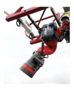
**WATER MONITOR:** When positioned at the tip, the water monitor can be elevated 30° higher than the elevation of the ladder.
