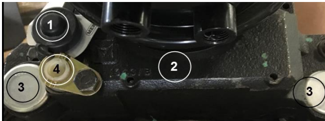
Meritor ADB rear view. 1- Adjuster cover. 2- Solid cast housing. 3- Slide pin caps. 4- Electronic wear sensor plug.
