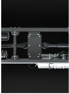
**PURPOSE-BUILT:** Pump placement is determined to ensure drive-line alignment and durability.
