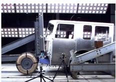
**TESTED TO NFPA CRASH STANDARDS:** *Third party tested including roof crush, front impact, and side impact testing to ensure the safety of our cabs.*
