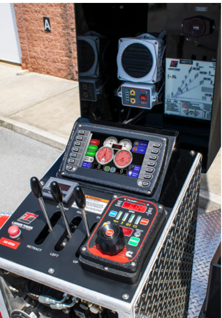
AL-11 AERIAL LOGIC: A totally integrated system that provides instant feedback on a ladder's extension, location, retraction, angle, load and breathing air system status, as well as J1939 engine information.
