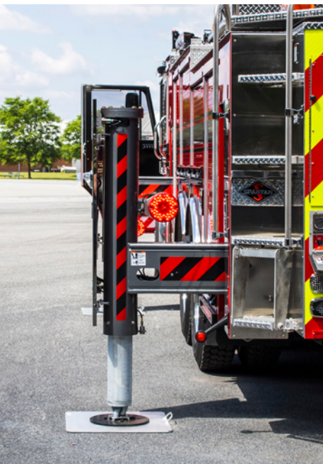
NARROW OUTRIGGER SPREAD: It's simple, if you can open your door you can set the jacks. A 12' outrigger spread with quick and simple deployment delivers industry leading performance.
