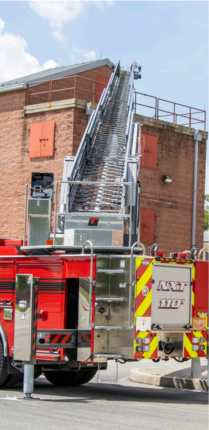
SAFE & EASY ACCESS: Wide egress steps and walkways provide easy access to and from the ladder.
