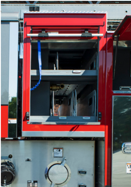
LOW CROSSLAYS: The low profile pump creates a safe and more ergonomic access to crosslays.
