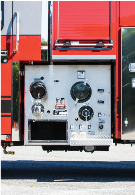
MAXIMUM PUMP CAPABILITIES: The non-proprietary NXT pump offers up to 2,250 GPM along with added room and storage in the cab and body.
