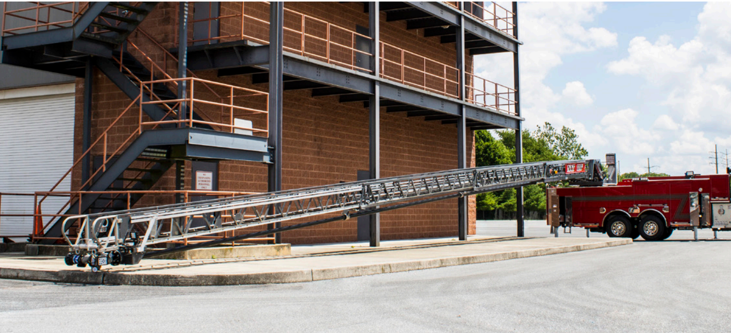
EXCELLENT HORIZONTAL & VERTICAL REACH: Built with up to 100,000 psi yield strength steel that can be depressed as low as 7° below horizontal or as high as 78° above horizontal. This allows firefighters to reach taller structures and have easy access to the ladder when lowered to ground level.
