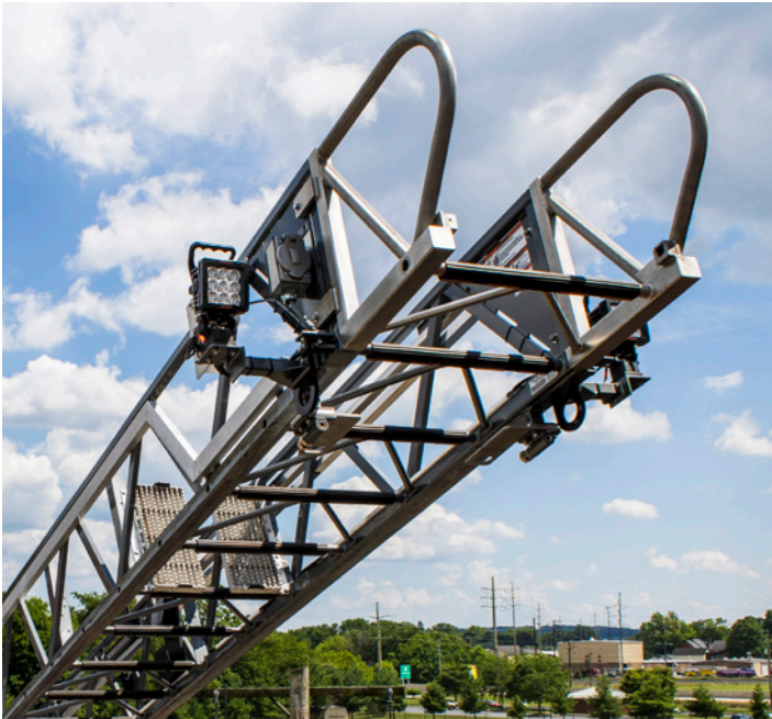
REPLACEABLE EGRESS: Designed with an unobstructed opening for easy access, the bolt-on removable egress can be easily replaced. Available in various lengths.
