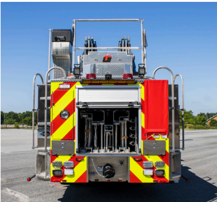
LOW GROUND LADDER STORAGE: Fully enclosed ground ladders are located just 40" from the ground, providing safe and ergonomic access to up to 170 ft. of storage.
