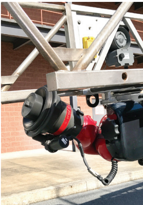
WATER MONITOR: When positioned at the tip, the water monitor can be elevated 30° higher than the elevation of the ladder.
