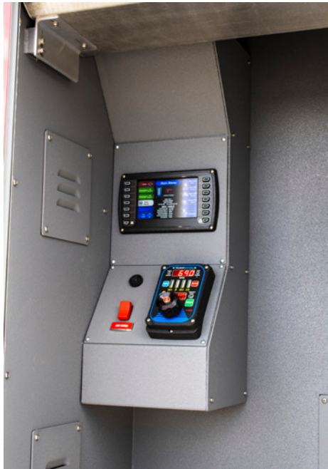
PUMP OPERATORS PANEL: The pump operators panel can be found inside the L2 compartment. Choose from standard controls or the optional Omni Pump System shown above.
