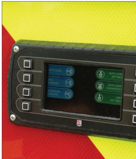
**SPARTAN SELF-LEVELING SYSTEM (SSL):** After the outriggers are deployed, the truck can be automatically leveled with a push of a button. The optional SSL system also stows the outriggers at the touch of a button. Available on Smeal aerials.
