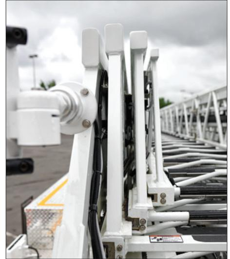
**LOWER TRAVEL HEIGHT:** Ladders stack efficiently, providing a low profile and lower travel heights, making it easy to fit into historic firehouses and under bridges. Available on Ladder Tower aerials.
