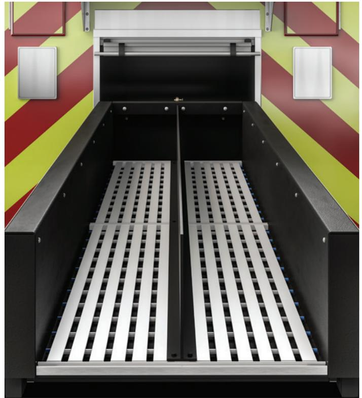
**ERGONOMIC HOSE LOAD (EHL):** *Our patented, heavy-duty, electric/hydraulic hose loader option improves crew safety by placing a maximum of 1,000 feet of 5" LDH within a firefighter's reach (lowers to 42" off the ground), eliminating climbs on a wet or slippery apparatus to reload hose. Available on Smeal Rear Mount aerials.*
