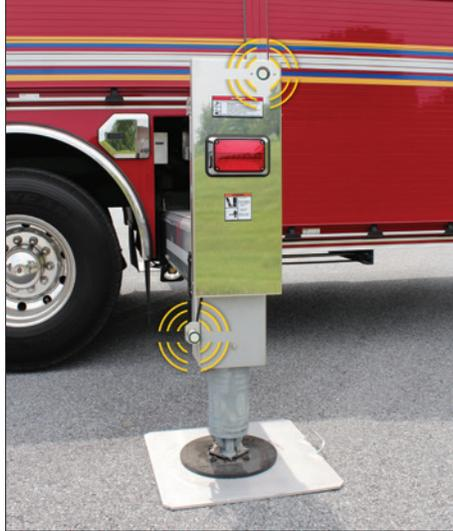
**OUTRIGGER DETECTION SYSTEM:** Automatically detects obstacles at scene to ensure secure placement of outriggers. Available on all models of aerials.
