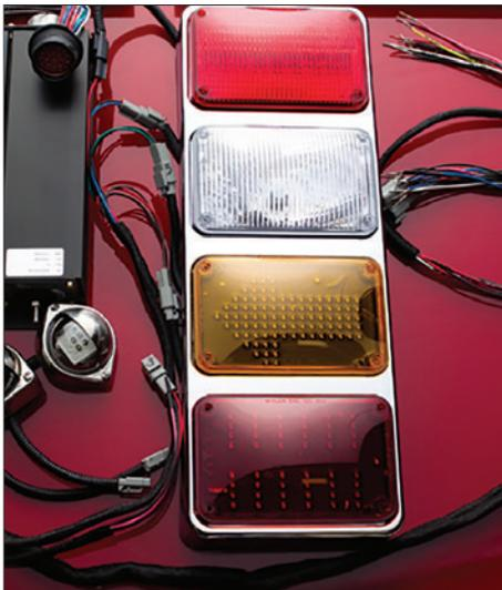
**QL-12 ELECTRICAL SYSTEM:** Our plug-and-play system reduces the amount of non-plug connectors and makes it easy to add components and make repairs to the electrical system. Available on Smeal aerials.
