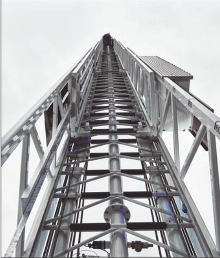
**RETRACTION OVERRIDE:** Retraction automatically stops as the steps on the fly section near overlapping with the next lower section; this ensures crew safety and prevents potential injury. Available on Smeal aerials.
