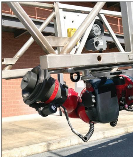
**WATER MONITOR:** When positioned at the tip, the water monitor can be set to reach 30° higher than the elevation of the ladder. Available on both brands and all models of straight aerials.
