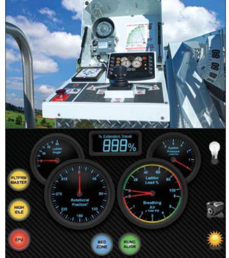
**AL-11 AERIAL LOGIC:** A totally integrated system that provides instant feedback on a ladder's extension, location, retraction, angle, load and breathing air system status, as well as J1939 engine information. Available on Smeal aerials.
