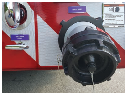
Figure 3-23. Waterway Drain and Aerial Inlet
