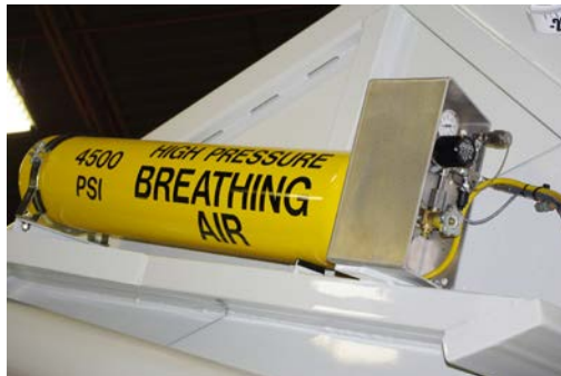
Figure 3-19. Breathing Air System High-Pressure Cylinder
