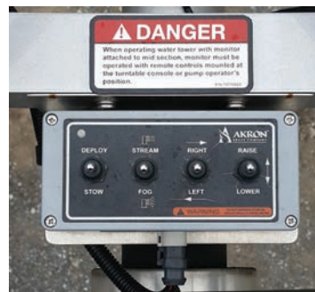
Figure 3-17. Monitor and nozzle control
