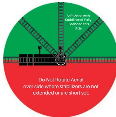
Figure 2-2. Short Set Rotation Interlock Stop Points
