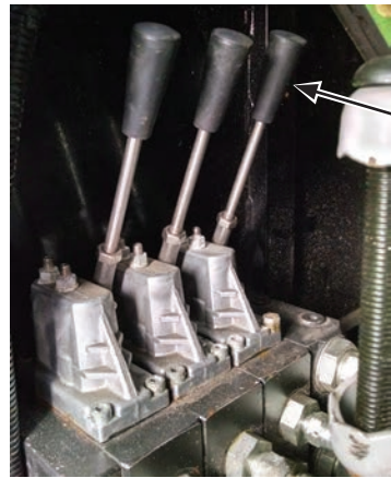
Figure 4-6. Manually Overriding the Snorkel Electric Controls
