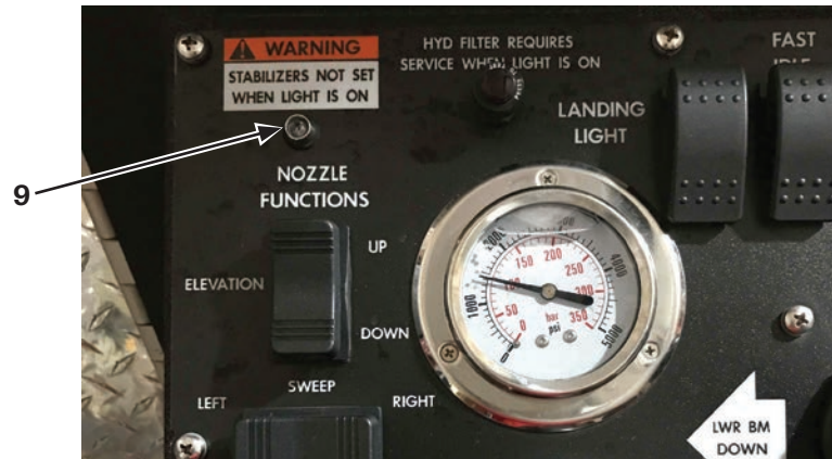
Figure 3-6. Stabilizer not set
