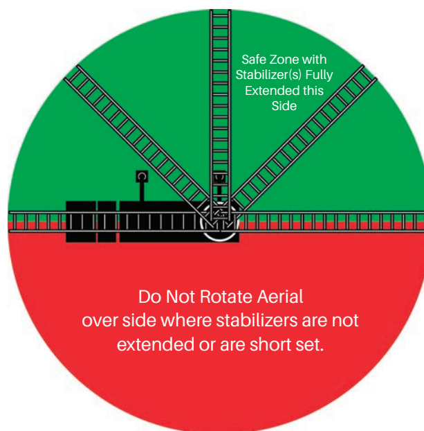
Figure 2-2. Short Set Rotation Interlock Stop Points
