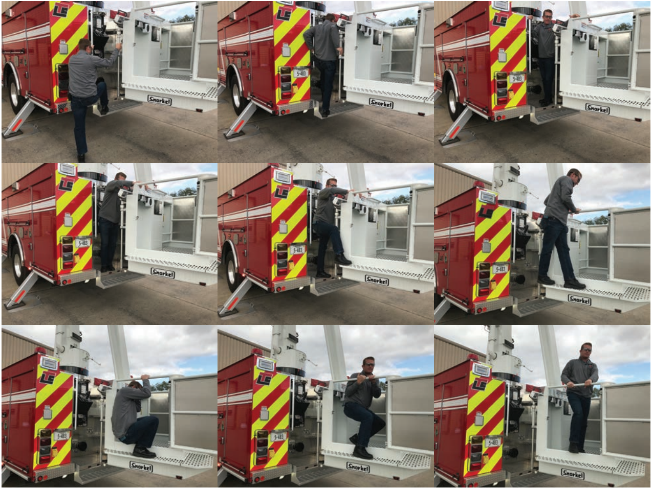
Figure 4-4. Platform Bucket Access Method
