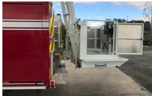
Figure 4-3. Device Orientation of Platform Bucket Access
