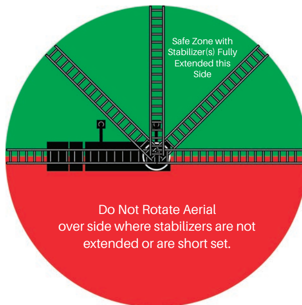
Figure 2-2. Short Set Rotation Interlock Stop Points
