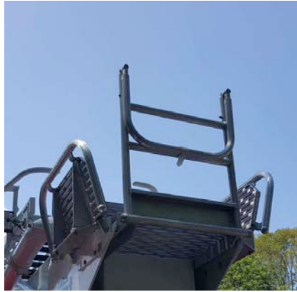
Figure 4-6. Handrail and platforms stowed
