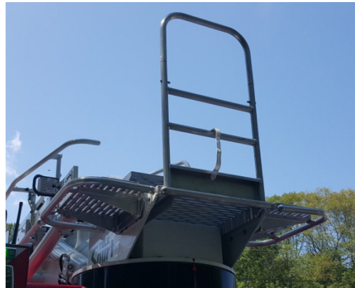
Figure 4-7. Handrail and platforms deployed
