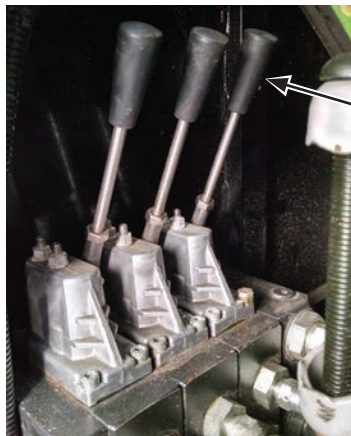
Figure 4-12. Manually Overriding the Telesqurt Boom Electric Controls
