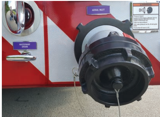
Figure 3-23. Waterway Drain and Aerial Inlet
