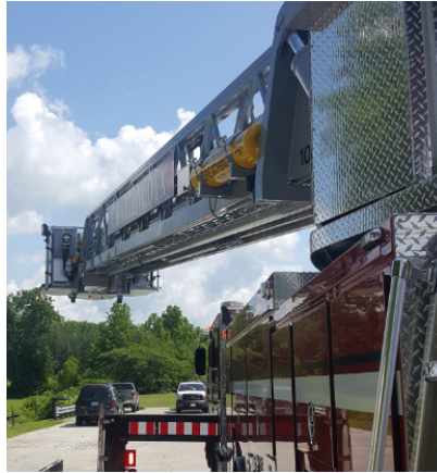
Figure 3-18. Ladder Movement Stops Prior to Contacting Body of Apparatus
