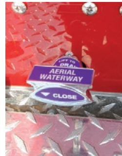
Figure 3-23. Waterway Drain and Aerial Inlet
