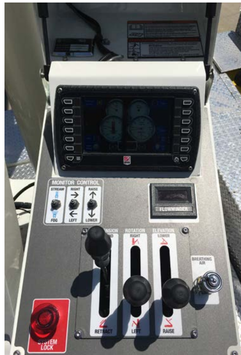
Figure 3-11. Primary Operator Control Station - AL-11
