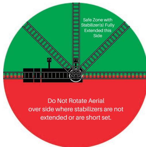
Figure 4-4. Short Set Rotation Interlock Stop Points
