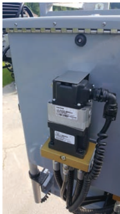
Figure 4-21. Manual Emergency Platform Bucket Leveling - Servo-Valve Control Under Cover
