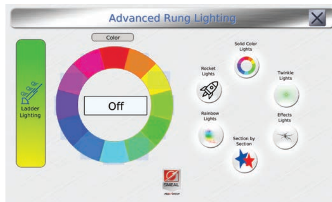
Figure 3-13. Advanced Rung Lighting Menu Screen
