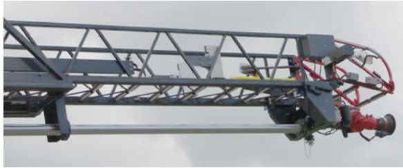
Figure 4-15. Monitor at the end of the Fly Section
