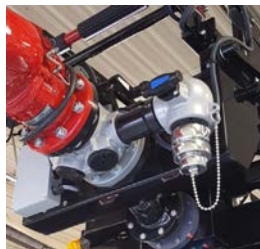
Figure 4-18. Aerial Standpipe Connection
