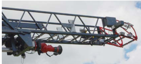
Figure 4-16. Monitor at the end of Next Lower Ladder Section
