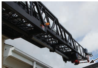
Figure 4-7. Maintain sufficient ladder clearance
