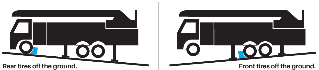
Figure 4-3. Leveling an Apparatus with 4 Stabilizers
