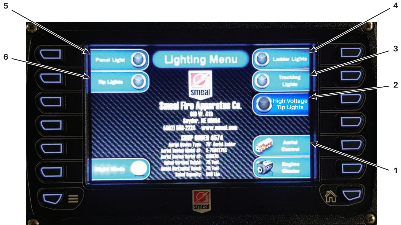
Figure 3-15. AL-11 Lighting Control Screen
