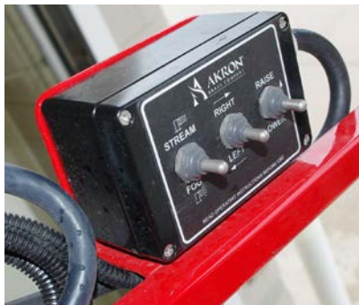
Figure 3-18. Monitor and nozzle control
