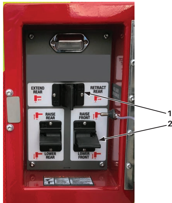
Figure 3-7. Stabilizer Controls - 2 Beams and 4 Jacks
