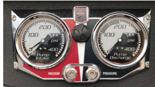
Figure 3-5. Master Discharge and Intake Pressure Gauges
