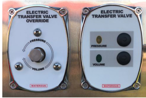
Figure 3-14. Pump Transfer Valve Control
