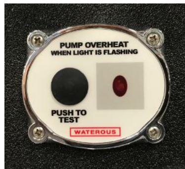
Figure 3-17. Pump Overheat Indicator
