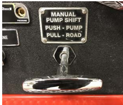
Figure 3-16. Manual Pump Shift Control
