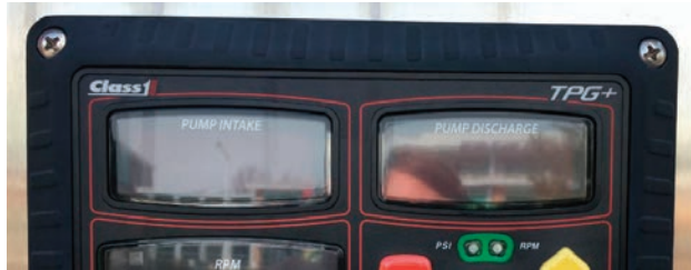
Figure 3-5. Master Discharge and Intake Pressure Gauges
