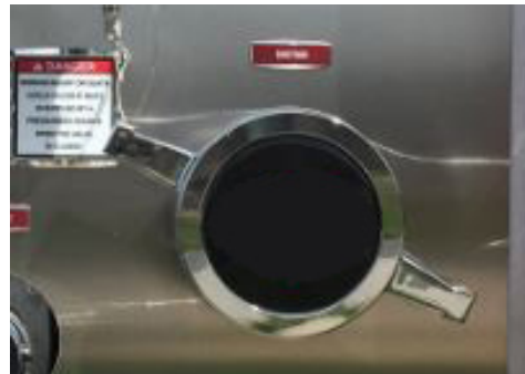
Figure 3-8. Steamer Intake Connection
