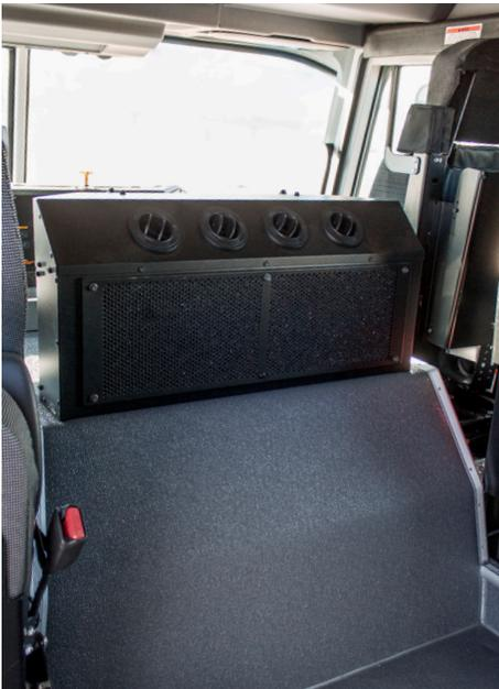
**CENTRAL A/C & HEAT:** Centrally located, the tunnel mount system is designed to deliver superior cooling and heating for the entire crew.
