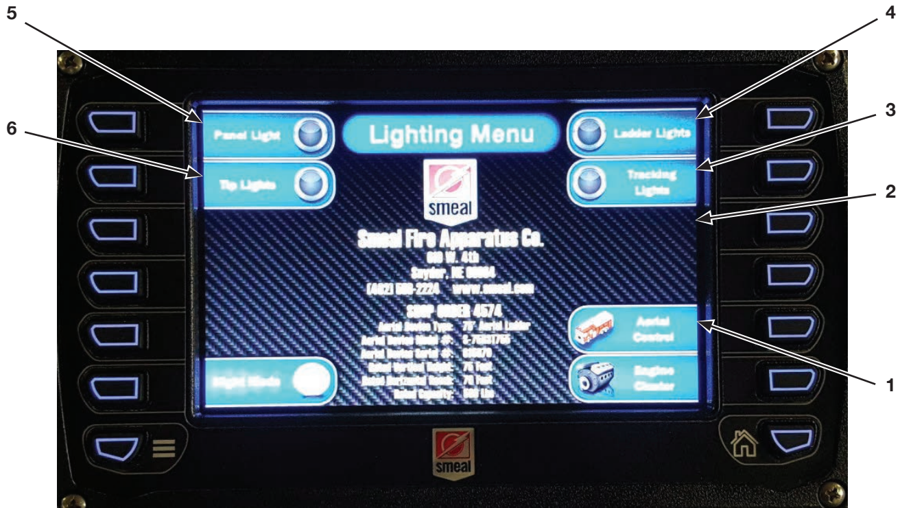
Figure 3-19. AL-11 Lighting Control Screen
