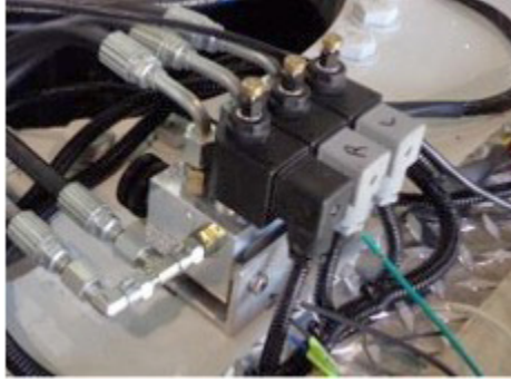
Figure 4-18. Rotation Override Valve Located Inside the Turntable Step to the Ladder
