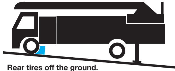
Figure 4-4. Leveling an Apparatus with 2 Stabilizers
