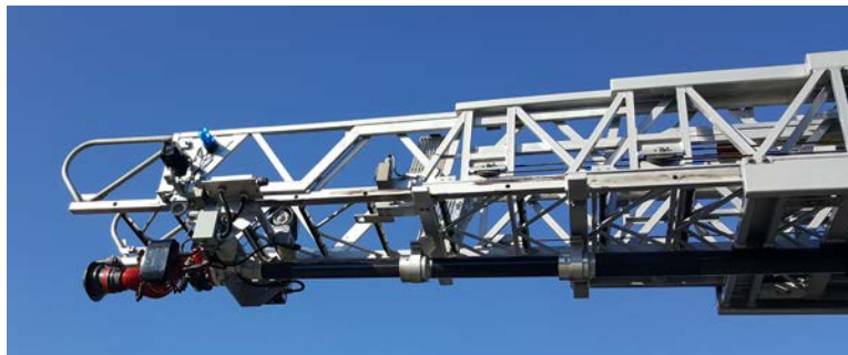
Figure 4-11. Monitor at the End of the Fly Section
