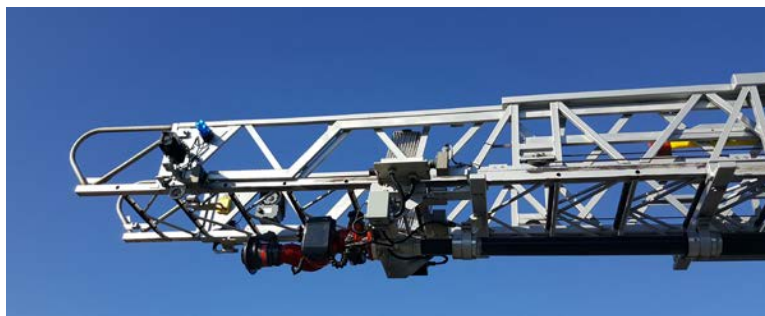
Figure 4-12. Monitor at the End of the Mid-Fly Section
