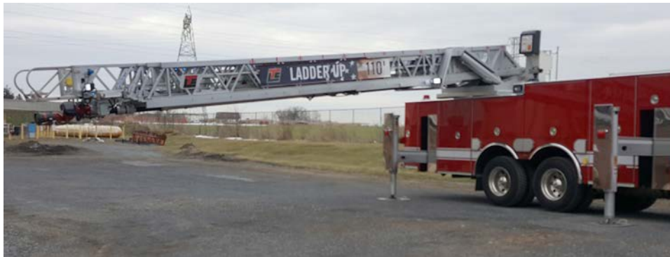
Figure 3-26. Ladder Movement Stops Prior to Contacting Body of Apparatus
