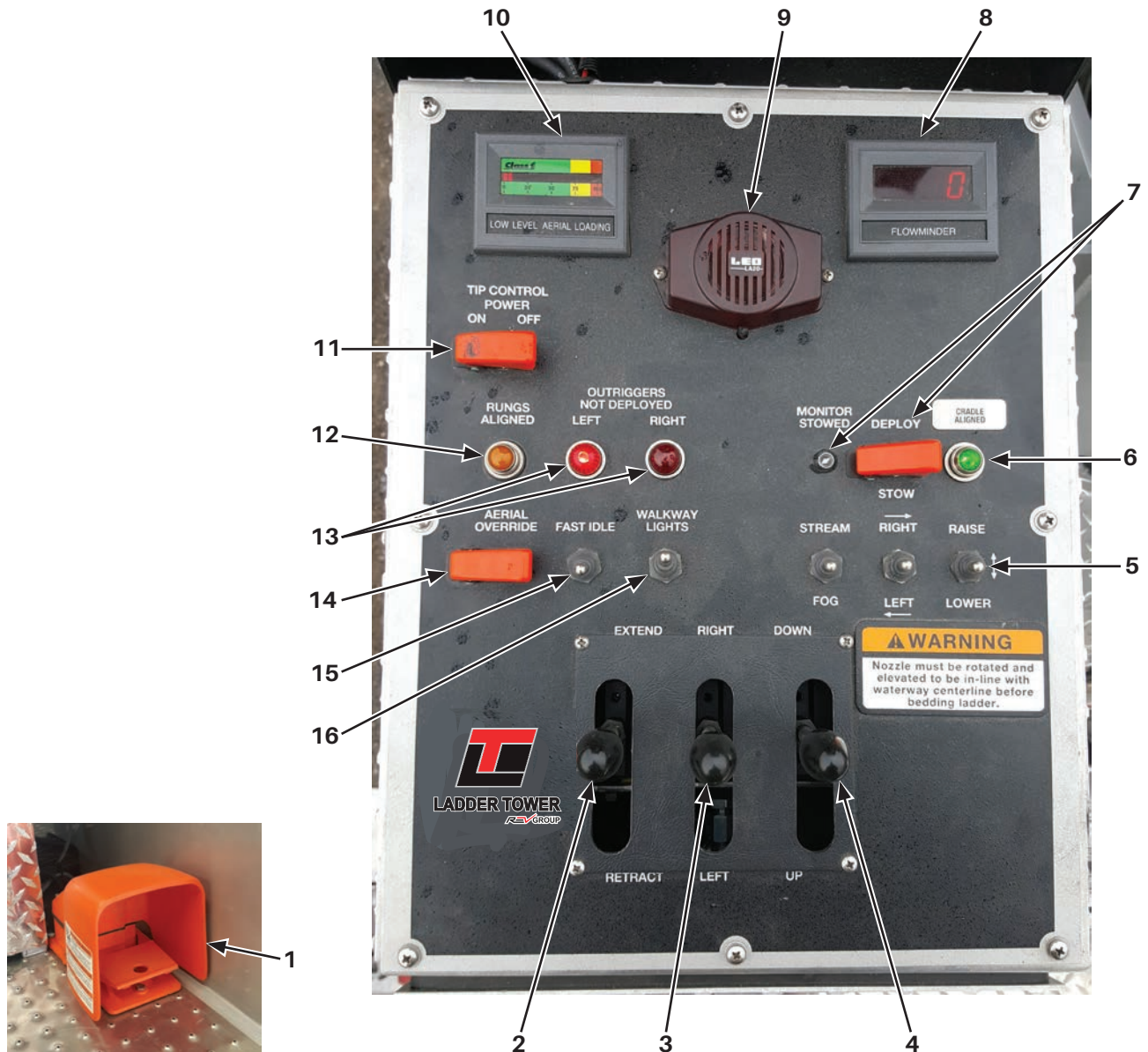
Figure 3-9. Primary Operator Control Station - Traditional
