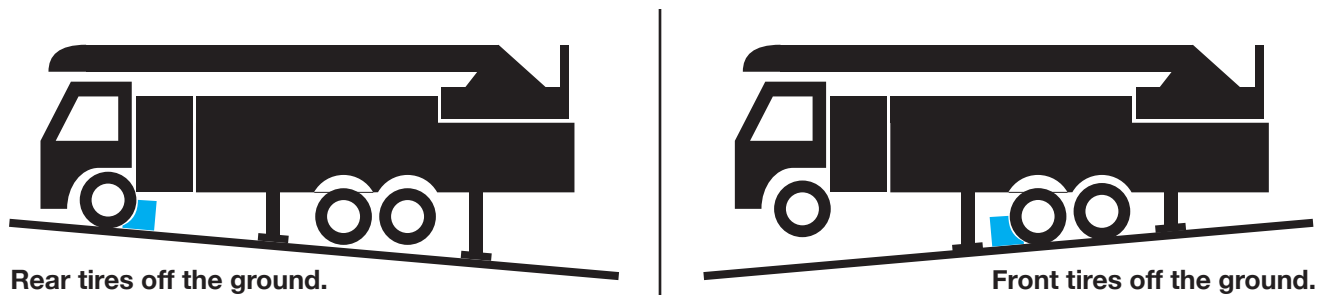
Figure 4-5. Leveling an Apparatus with 4 Stabilizers
