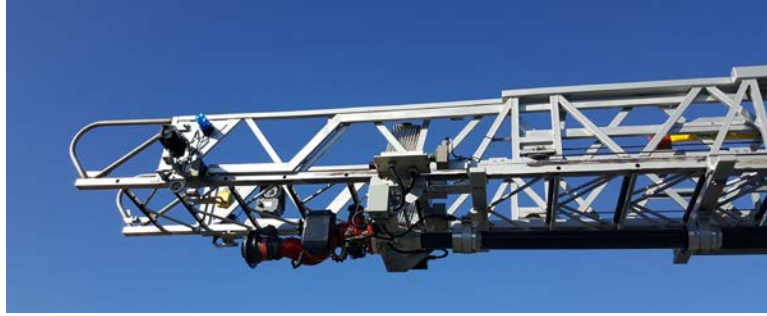
Figure 4-13. Monitor at the End of the Mid-Fly Section
