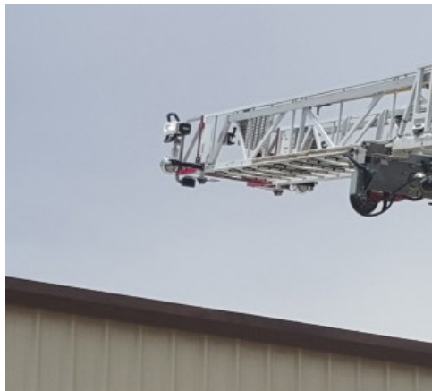
Figure 4-7. Maintain sufficient ladder clearance
