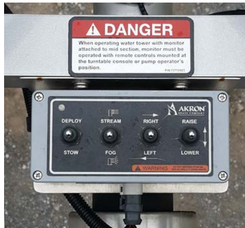
Figure 3-21. Monitor and Nozzle Control
