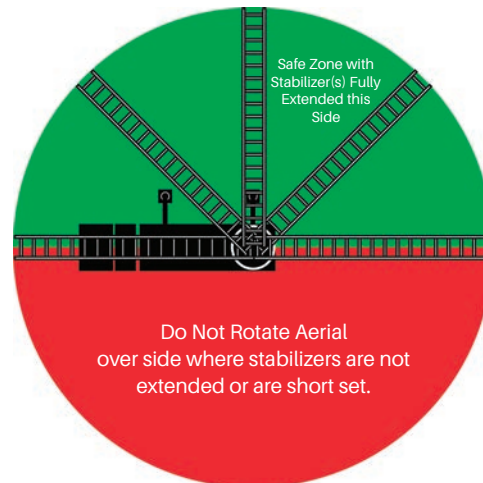
Figure 2-2. Short Set Rotation Interlock Stop Points
