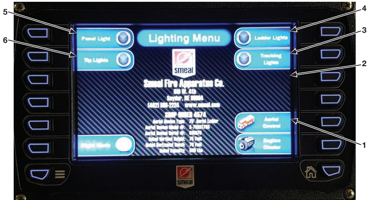
Figure 3-19. AL-11 Lighting Control Screen
