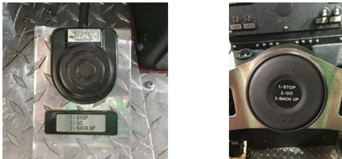
Figure 3-28. 1-2-3 Stop/Go/Backup Switches - Foot Switch and Steering Wheel Switch
