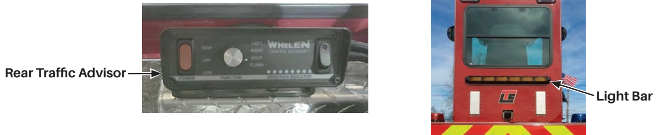
Figure 3-30. Tiller Trailer Rear Traffic Advisor Control and Light Bar
