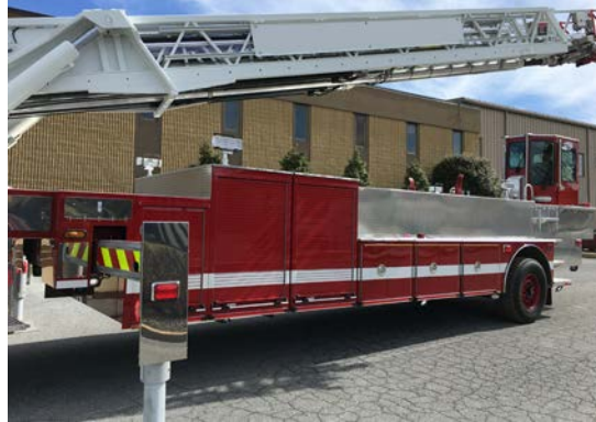
Figure 3-24. Ladder Movement Stops Prior to Contacting Body of Apparatus
