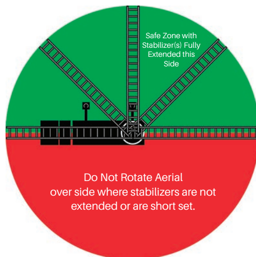
Figure 4-5. Short Set Rotation Interlock Stop Point
