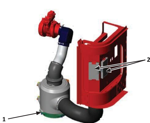
Typical Air Intake System – Conventional
